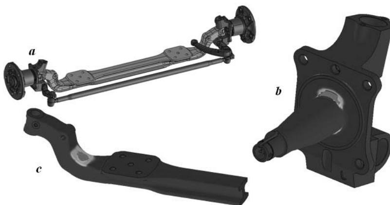
FIG. 2 – Assembly model and fatigue damage plot for axle assembly: a – 3D assembly model; b – fatigue damage plot of steering knuckle in case of stationary vertical loading; c – fatigue damage plot of axle in case of spectrum SAESUS loading.
